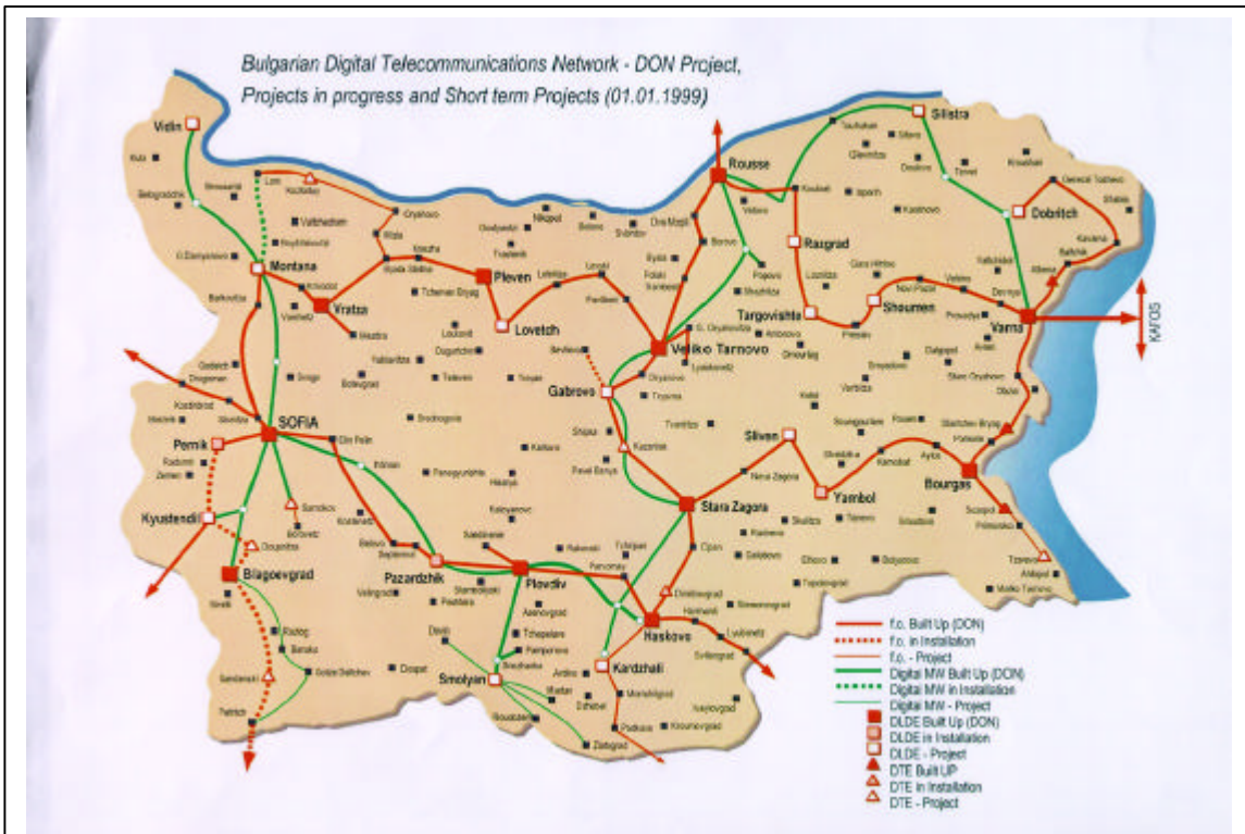
Figure 3: BTC's Analog and Digital Overlay Networks
